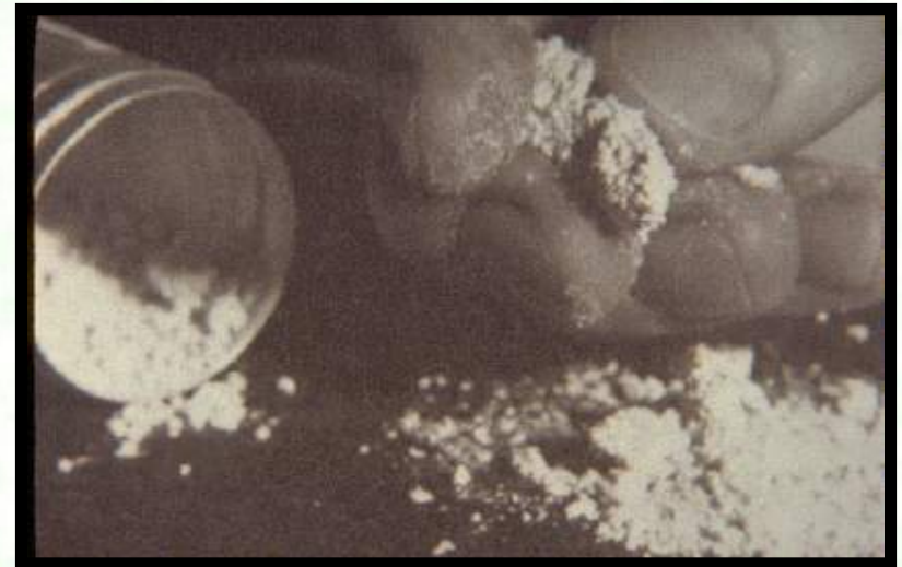
Photo of friable asbestos
